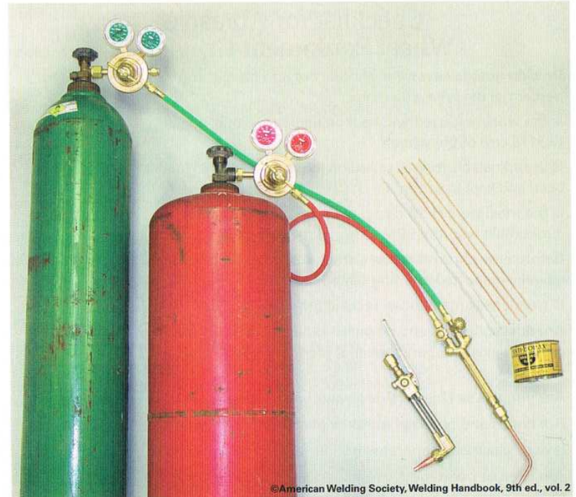
Oxy-fuel welding equipment
