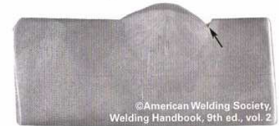
Undercut at the toe of an oxy-fuel arc weld
