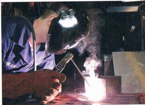
Welding beads with shielded metal arc welding
