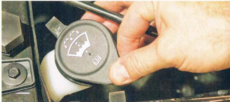
Windshield-washer fluid goes in a reservoir beneath a cap displaying a windshield wiper icon. The fluid includes detergent to clean the windshield and antifreeze to keep it from freezing in cold weather.
