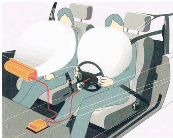
Air bags deploy automatically when a frontal crash occurs.
