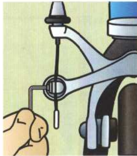
To adjust your brake cables, loosen the anchor bolt.
