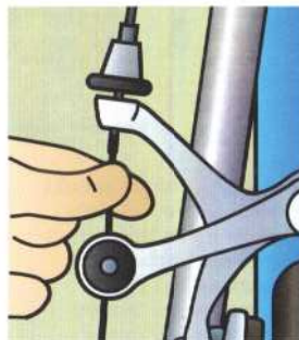
Tighten the anchor bolt. Then check the tension and readjust, if necessary.
