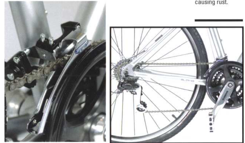
A good time to inspect the drive train and the rest of the bike for worn or broken parts is right after it has been cleaned.
