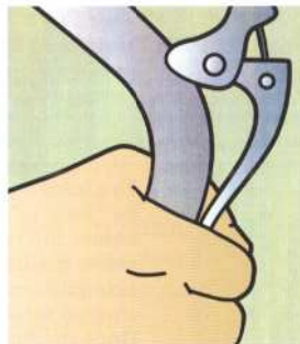
After the brakes are centered, check the whole brake system by squeezing the lever several times to see that the parts work promptly, nothing slips, and everything returns to a natural position when the levers are released.
