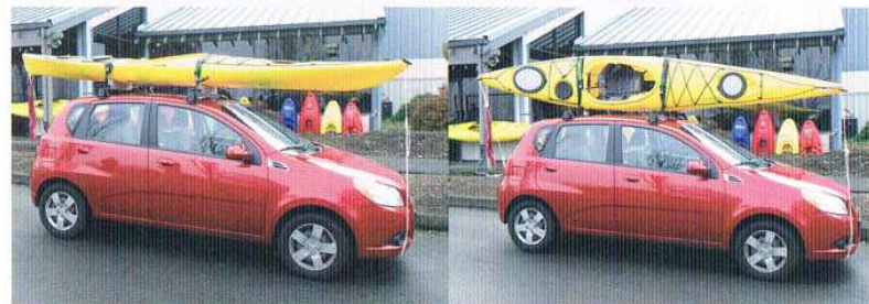
Tying on to a horizontal rack.
